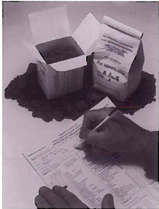
Figure 5. Thoroughly mix the air-dried sample, fill the sample bag or box, mark with your sample designation, fill out the information sheet, and take the sample to your county Extension office.
